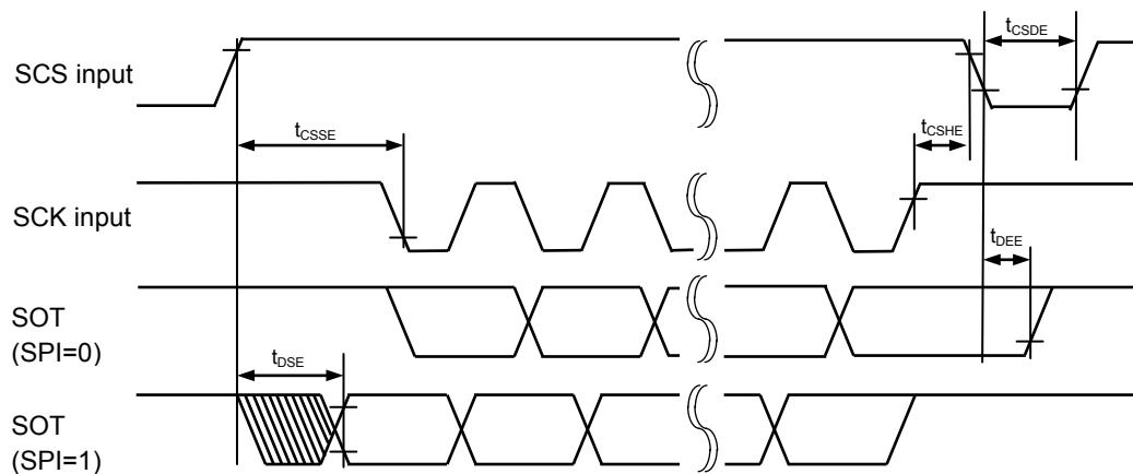
When Serial chip select is used , Serial clock output mark level "H",
