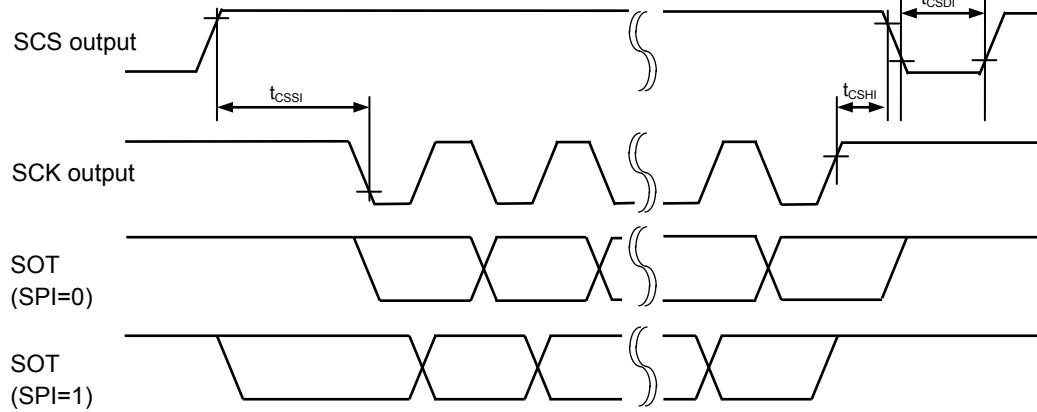
When Serial chip select is used , Serial clock output mark level "H",
