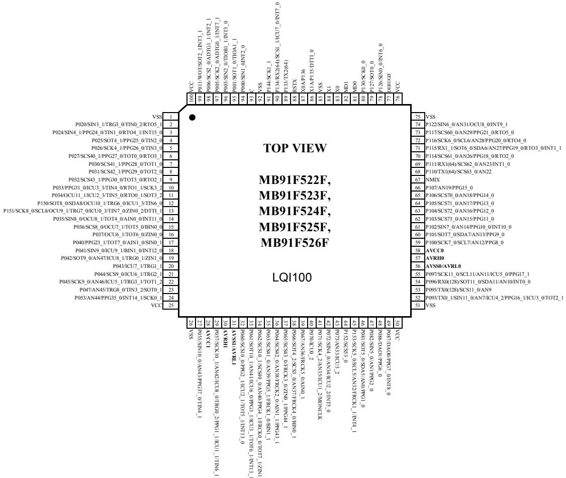
\* In a single clock product, pin 86 and pin 87 are the general-purpose ports.
