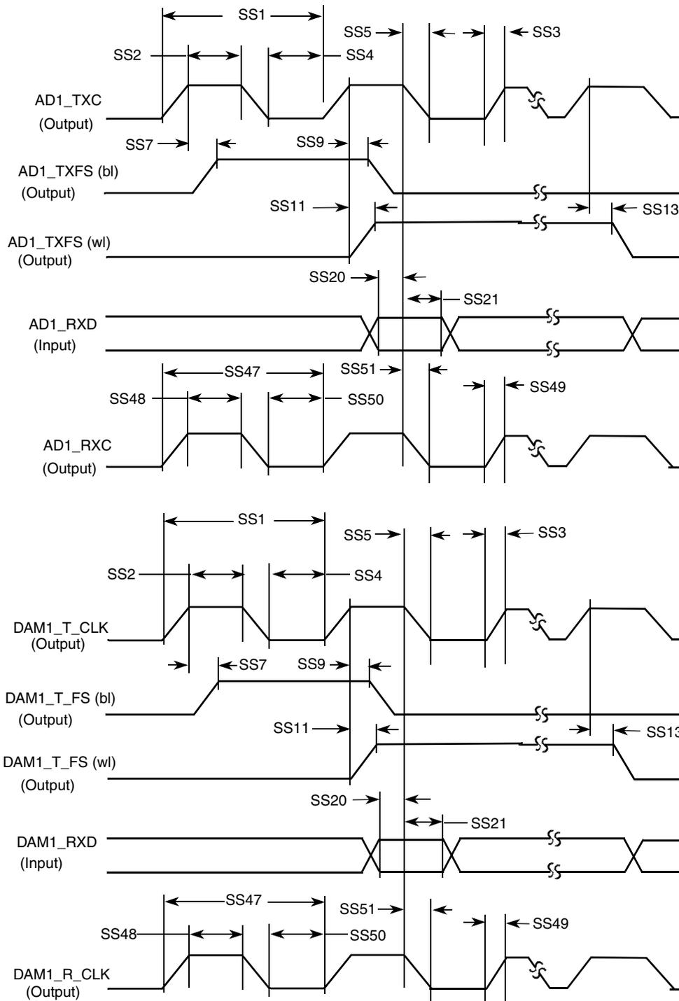
Figure 82. SSI Receiver with Internal Clock Timing Diagram
