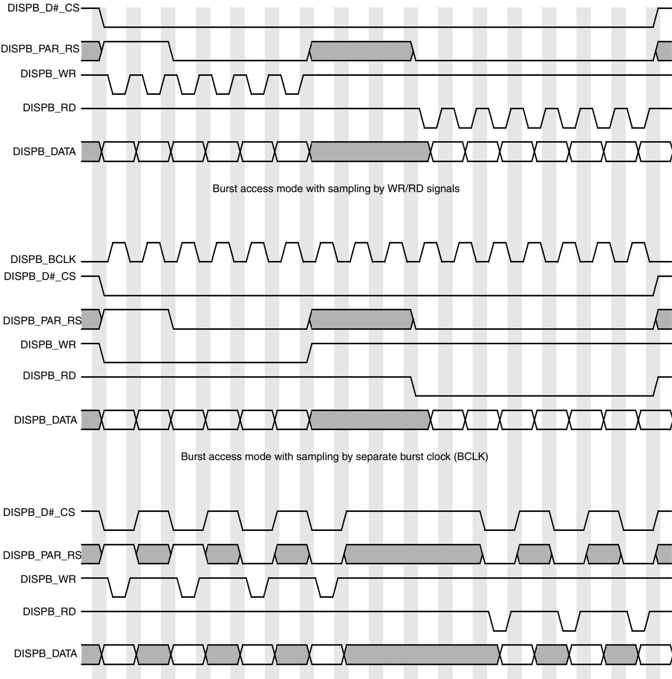
Single access mode (all control signals are not active for one display interface clock after each display access)
