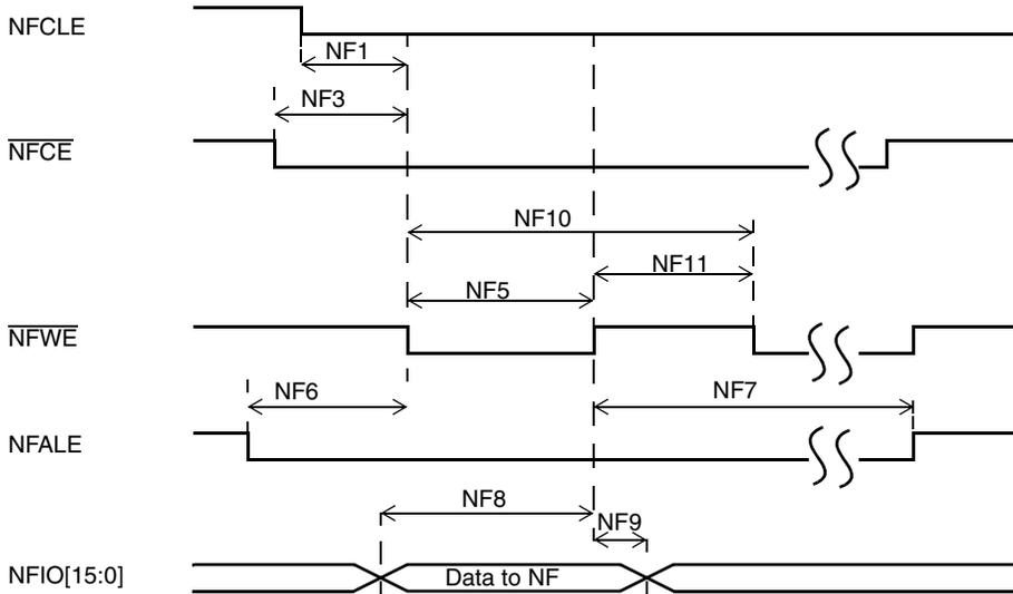
**Figure 25. Write Data Latch Cycle Timing Diagram**
