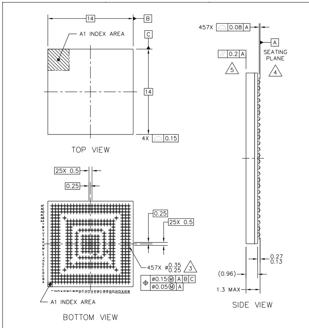
Figure 86. Production Package: Case 1581—0.5 mm Pitch
