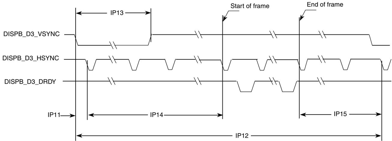
**Figure 48. TFT Panels Timing Diagram—Vertical Sync Pulse**
