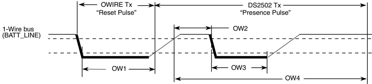
Figure 7. Reset and Presence Pulses (RPP) Timing Diagram
