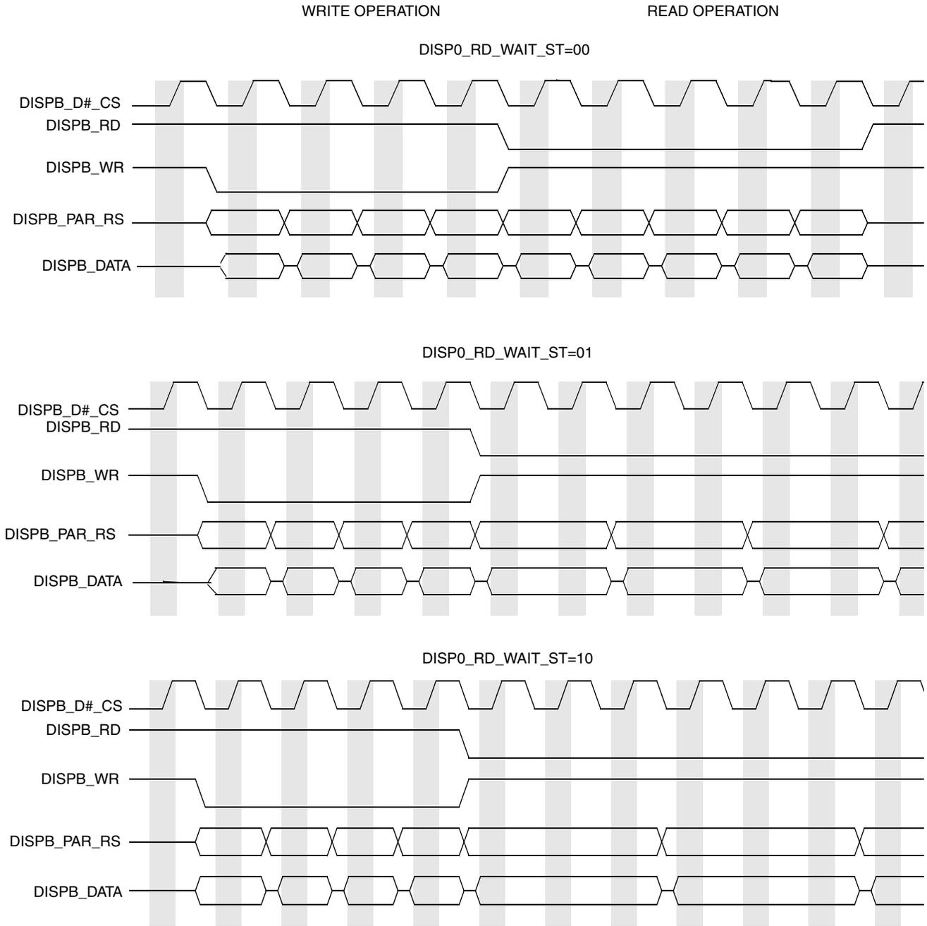
Figure 56. Parallel Interface Timing Diagram—Read Wait States
