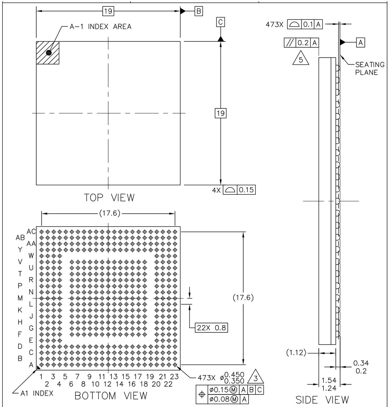
Figure 87. Production Package: Case 1931—0.8 mm Pitch
