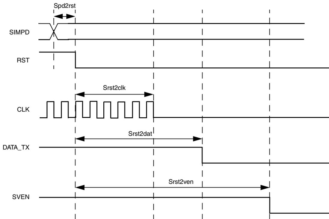
Figure 76. SmartCard Interface Power Down AC Timing
