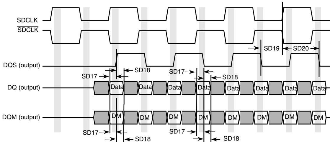
**Figure 38. Mobile DDR SDRAM Write Cycle Timing Diagram**
