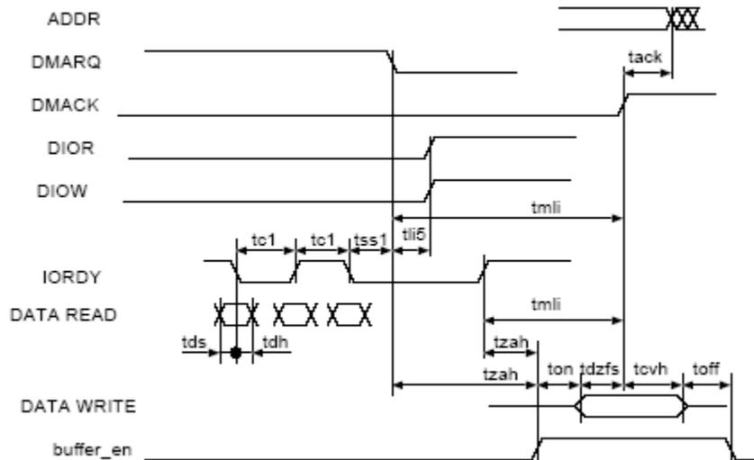
Figure 17. UDMA In Device Terminates Transfer Timing Diagram
