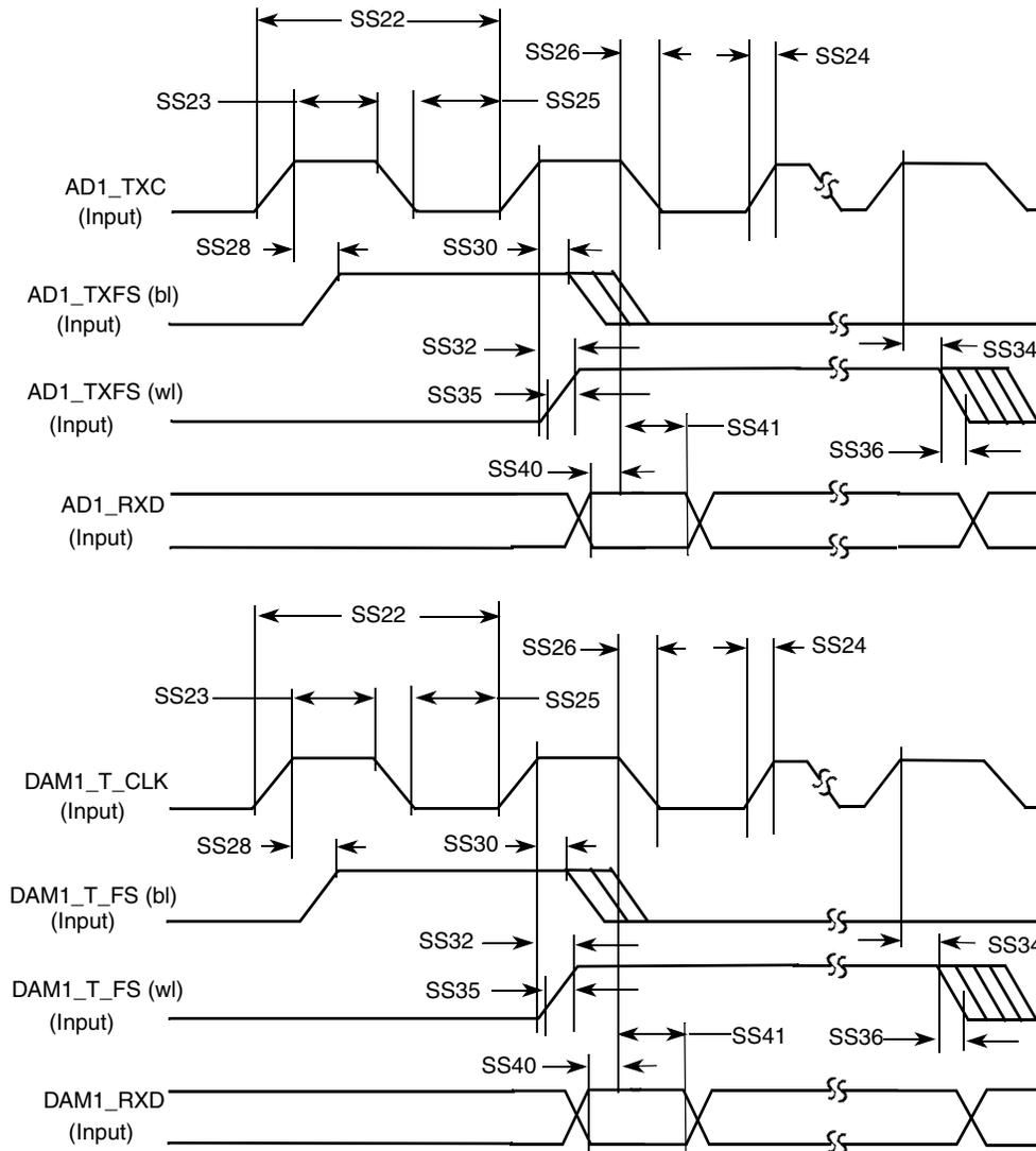
Figure 84. SSI Receiver with External Clock Timing Diagram
