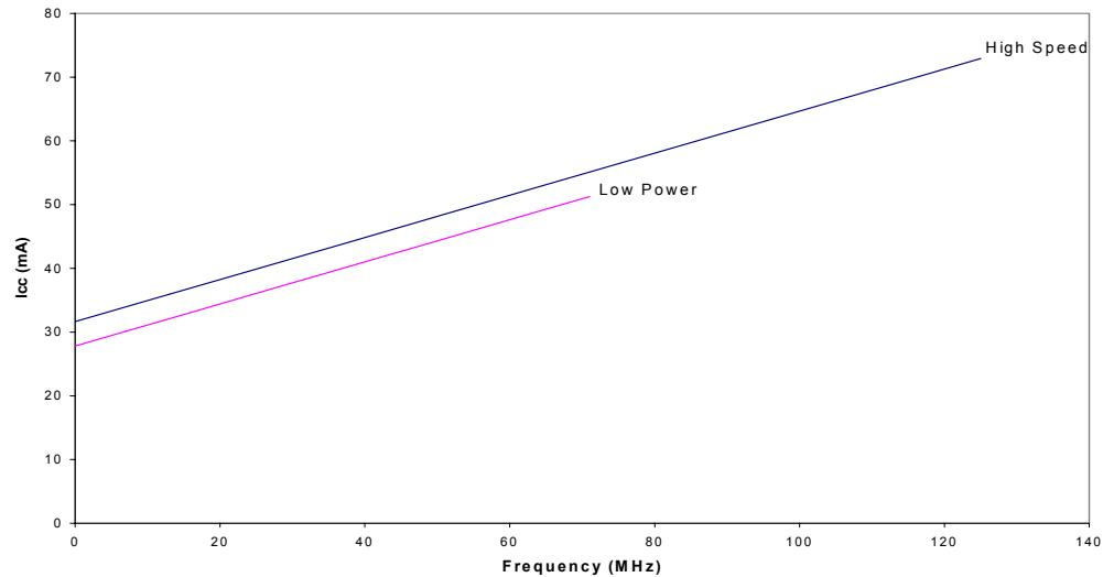
The typical pattern is a 16-bit up counter, per logic block, with outputs disabled.
