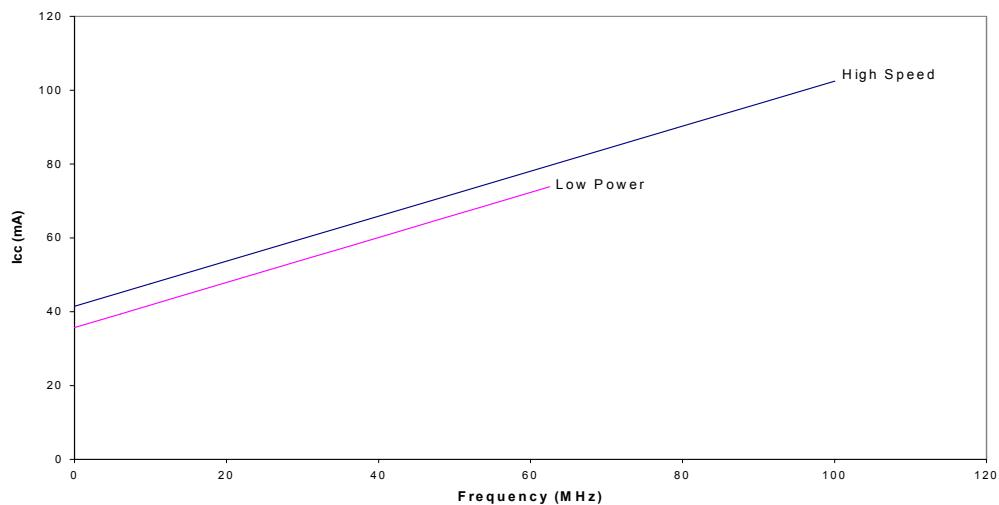
The typical pattern is a 16-bit up counter, per logic block, with outputs disabled.
