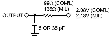
**3.3V AC Test Loads and Waveforms**
