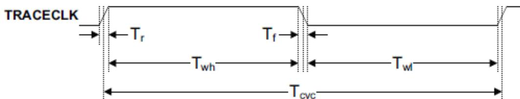
Figure 4. TRACE\_CLKOUT specifications
