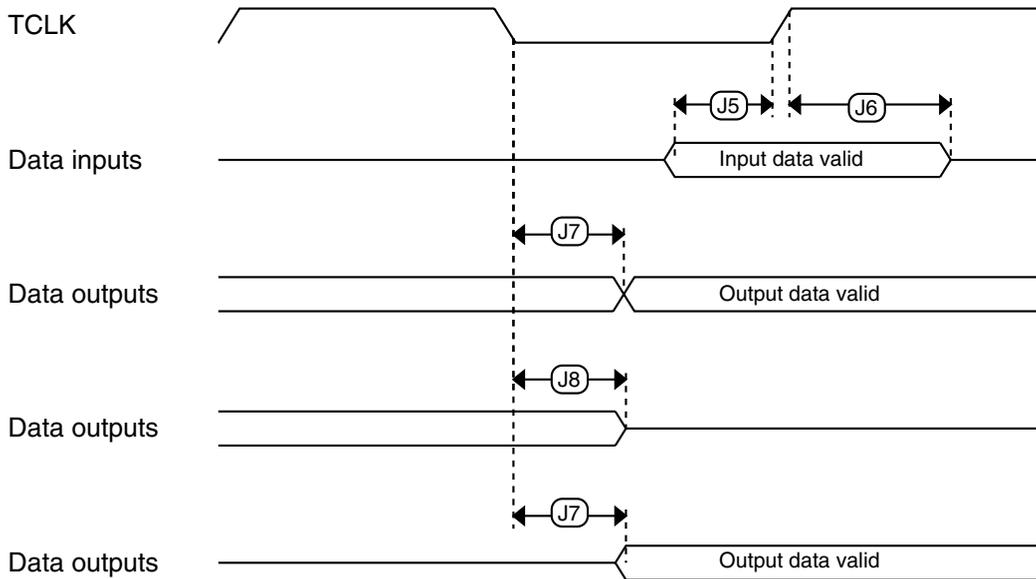
**Figure 7. Boundary scan (JTAG) timing**
