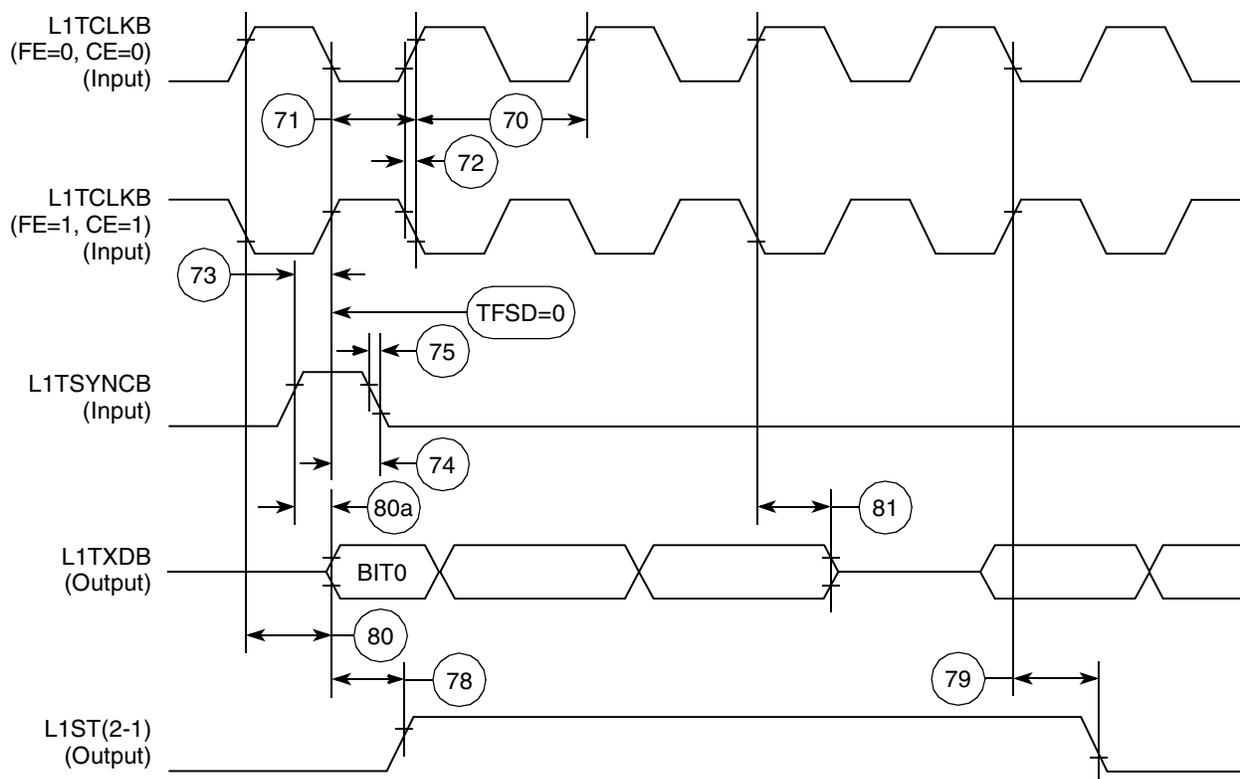
Figure 48. SI Transmit Timing Diagram (DSC = 0)
