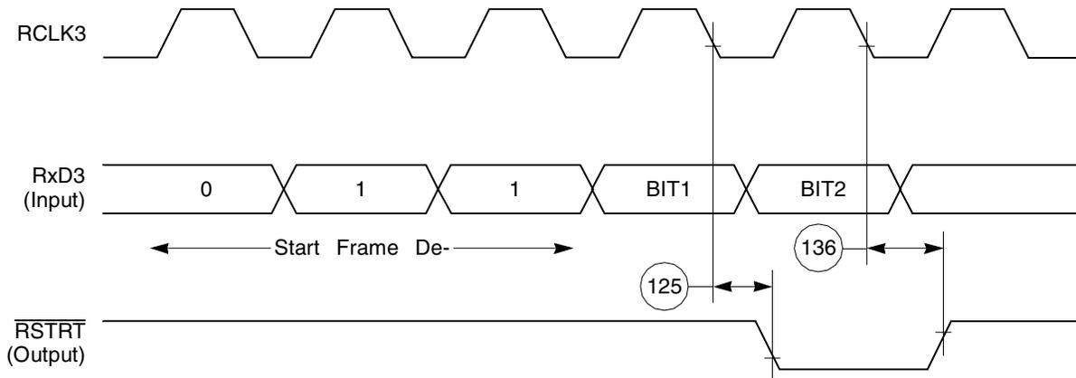
**Figure 57. CAM Interface Receive Start Timing Diagram**
