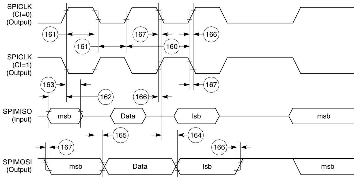
**Figure 59. SPI Master (CP = 0) Timing Diagram**
