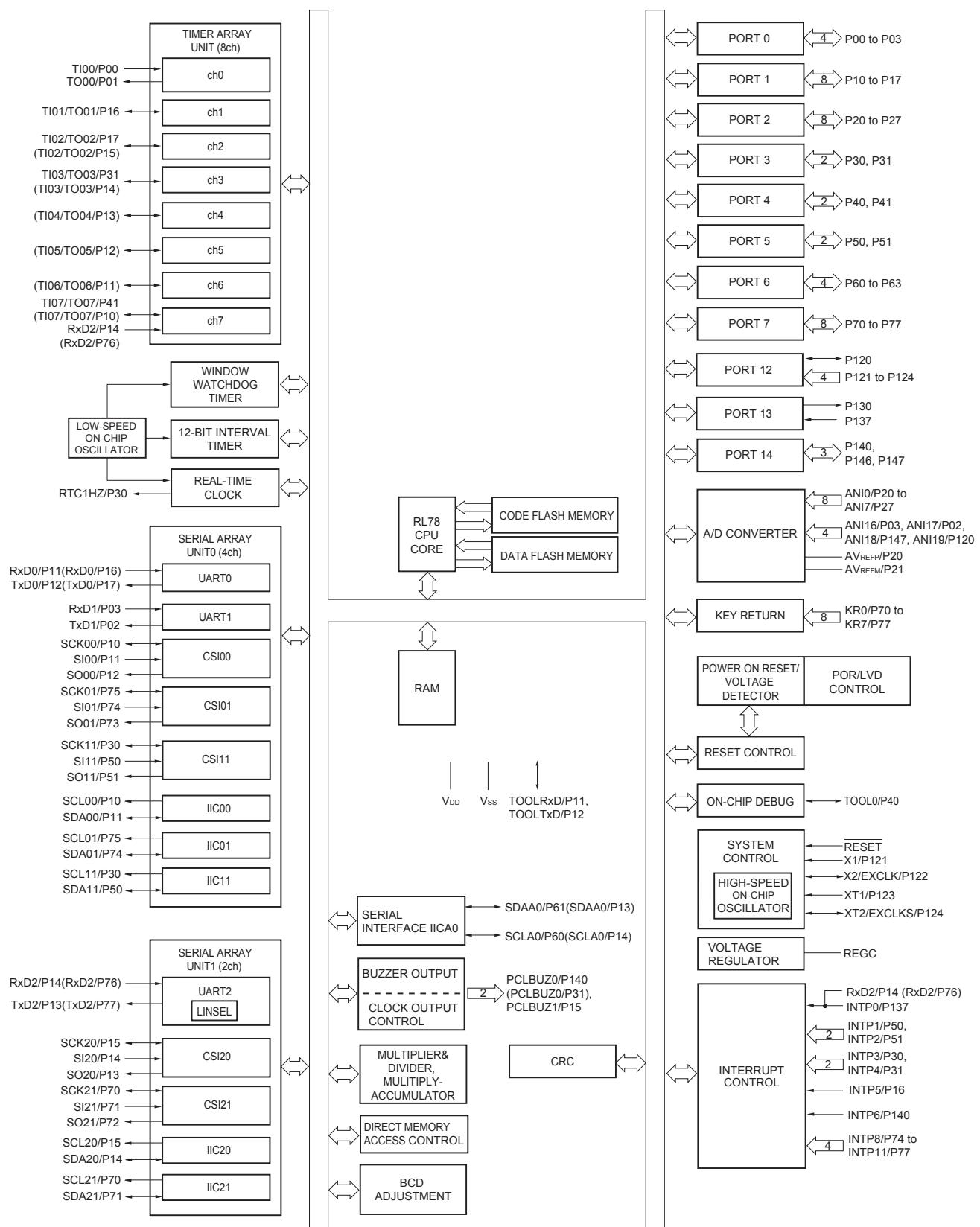
**Remark** Functions in parentheses in the above figure can be assigned via settings in the peripheral I/O redirection register (PIOR). Refer to **Figure 4-8 Format of Peripheral I/O Redirection Register (PIOR)** in the RL78/G13 User's Manual.
