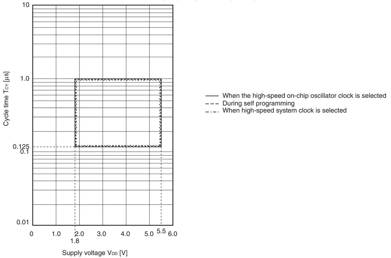
T<sub>CY</sub> vs V<sub>DD</sub> (LV (low-voltage main) mode)
