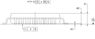
Each lead centerline is located within 0.08 mm of its true position at maximum material condition.
