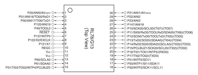
Caution Connect the REGC pin to Vss via a capacitor (0.47 to 1  $\mu$ F).
