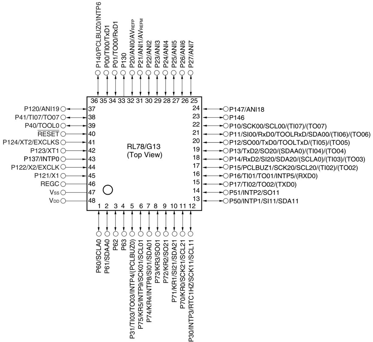
**Caution** Connect the REGC pin to V<sub>SS</sub> via a capacitor (0.47 to 1 μF).
