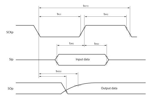
CSI mode serial transfer timing (slave mode) (during communication at different potential) (When DAPmn = 0 and CKPmn = 0, or DAPmn = 1 and CKPmn = 1.)
