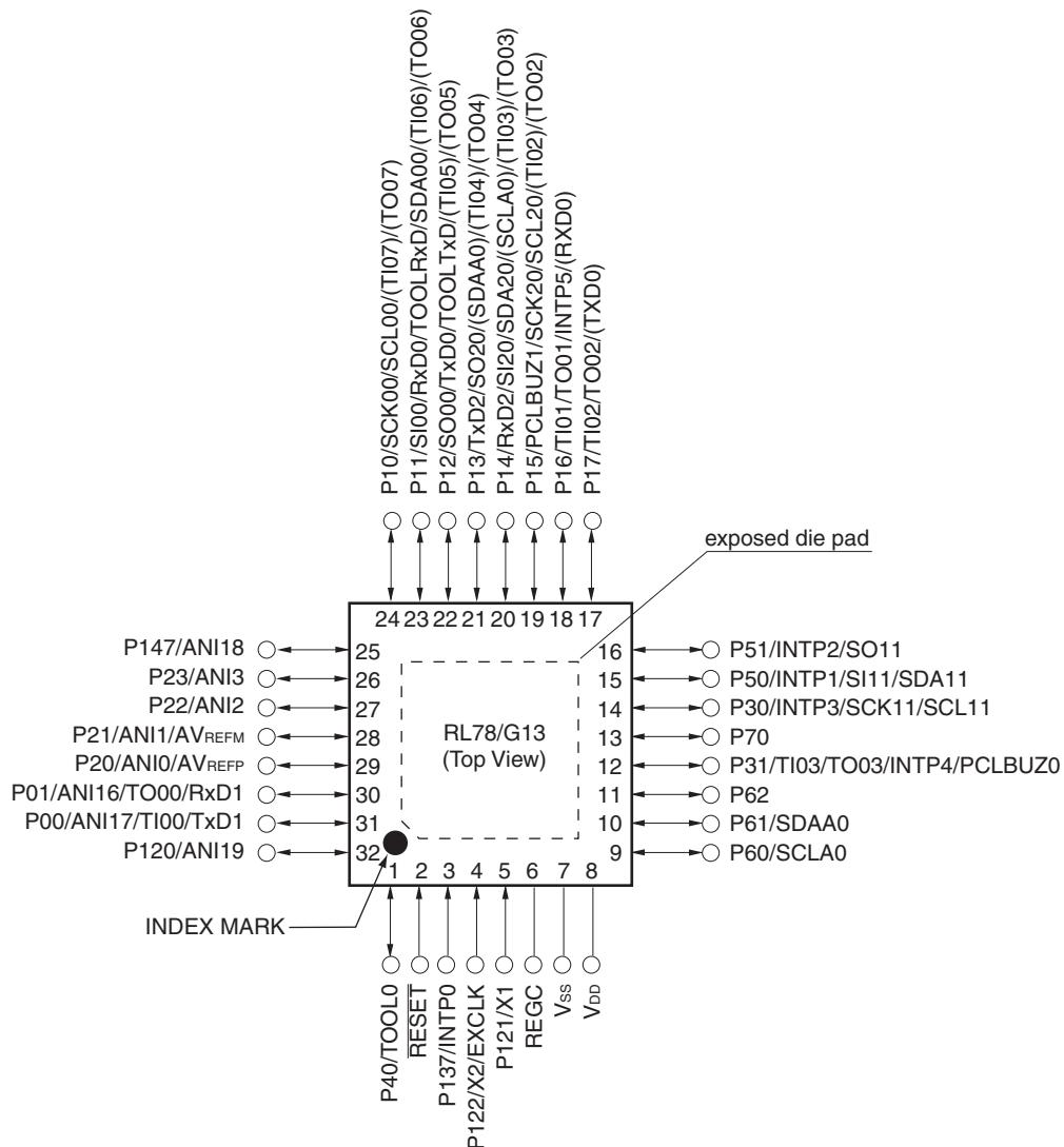
**Caution Connect the REGC pin to V<sub>ss</sub> via a capacitor (0.47 to 1  $\mu$ F).**
