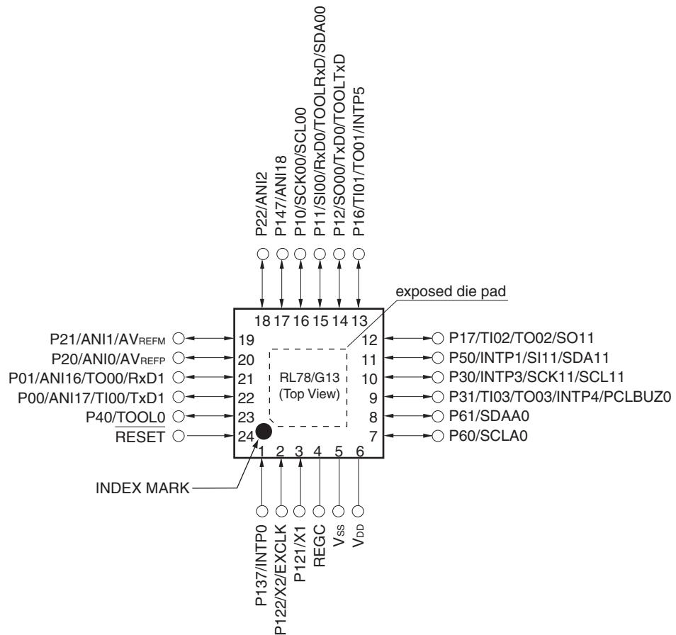
**Caution Connect the REGC pin to V<sub>ss</sub> via a capacitor (0.47 to 1  $\mu$ F).**
