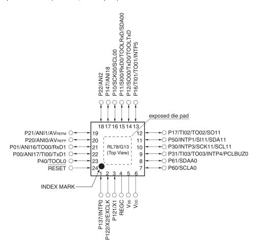
Caution Connect the REGC pin to Vss via a capacitor (0.47 to 1  $\mu$ F).
