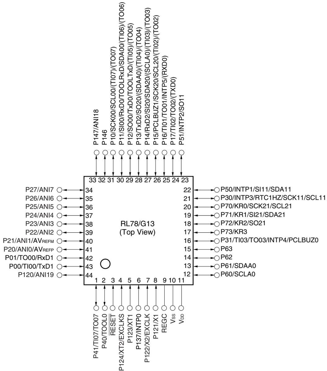
**Caution** Connect the REGC pin to V<sub>SS</sub> via a capacitor (0.47 to 1 μF).
