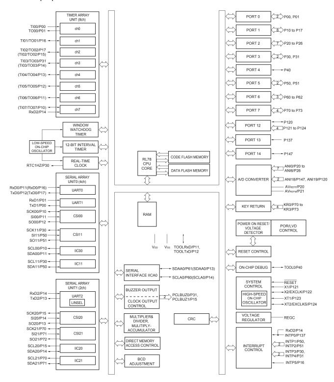
Remark Functions in parentheses in the above figure can be assigned via settings in the peripheral I/O redirection register (PIOR). Refer to Figure 4-8 Format of Peripheral I/O Redirection Register (PIOR) in the RL78/G13 User's Manual.
