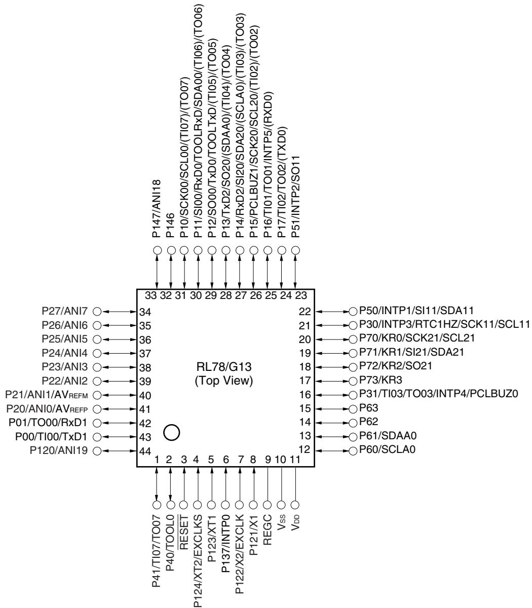
**Caution** Connect the REGC pin to Vss via a capacitor (0.47 to 1  $\mu$ F).
