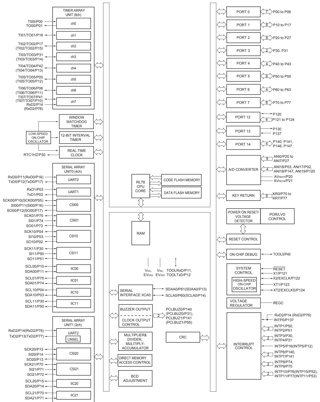
**Remark** Functions in parentheses in the above figure can be assigned via settings in the peripheral I/O redirection register (PIOR). Refer to **Figure 4-8 Format of Peripheral I/O Redirection Register (PIOR)** in the RL78/G13 User's Manual.
