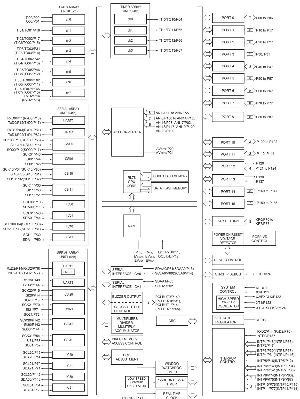
**Remark** Functions in parentheses in the above figure can be assigned via settings in the peripheral I/O redirection register (PIOR). Refer to **Figure 4-8 Format of Peripheral I/O Redirection Register (PIOR)** in the RL78/G13 User's Manual.
