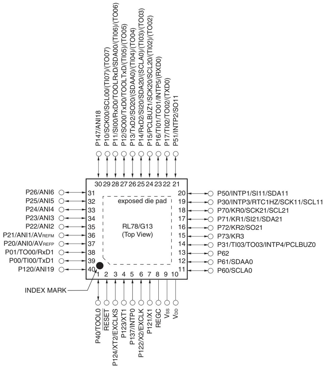
**Caution** Connect the REGC pin to V<sub>SS</sub> via a capacitor (0.47 to 1 μF).
