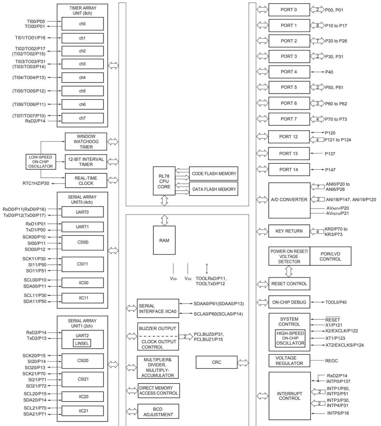
**Remark** Functions in parentheses in the above figure can be assigned via settings in the peripheral I/O redirection register (PIOR). Refer to **Figure 4-8 Format of Peripheral I/O Redirection Register (PIOR)** in the RL78/G13 User's Manual.
