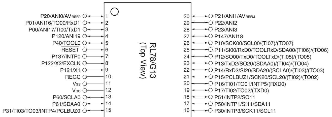
**Caution** Connect the REGC pin to V<sub>SS</sub> via a capacitor (0.47 to 1  $\mu$ F).
