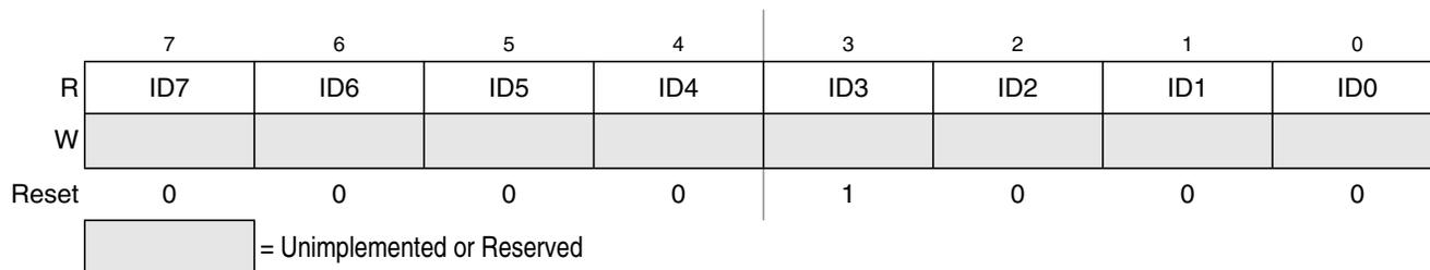
**Figure 5-8. System Device Identification Register — Low (SDIDL)**
