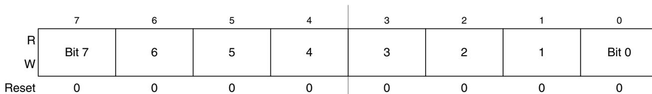
**Figure 10-10. Timer Channel Value Register Low (TPMxCnVL)**
