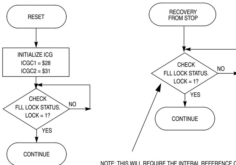
Figure 8-16. ICG Initialization and Stop Recovery for Example #3
