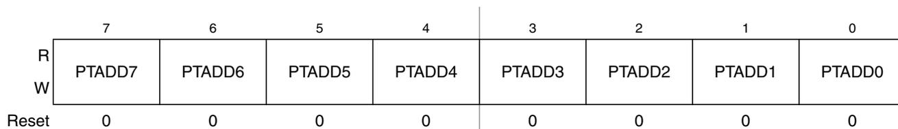
**Figure 6-10. Data Direction for Port A Register (PTADD)**
