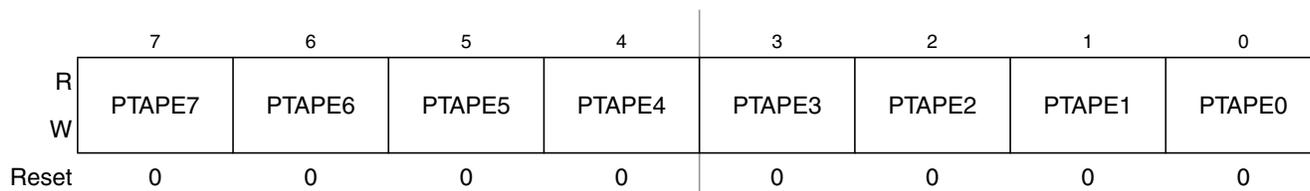
**Figure 6-11. Internal Pullup Enable for Port A (PTAPE)**
