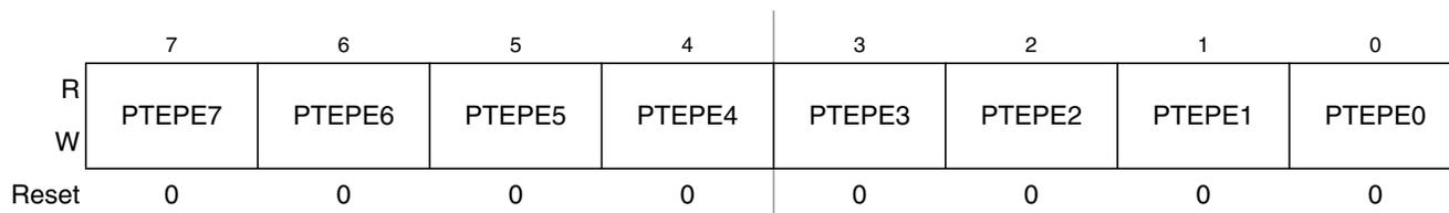
Figure 6-31. Internal Pullup Enable for Port E (PTEPE)
