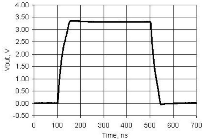
**Figure 11-24. USBIO Output Rise and Fall Times, GPIO Mode,  $V_{DD} = 3.3\text{ V}$ , 25 pF Load**
