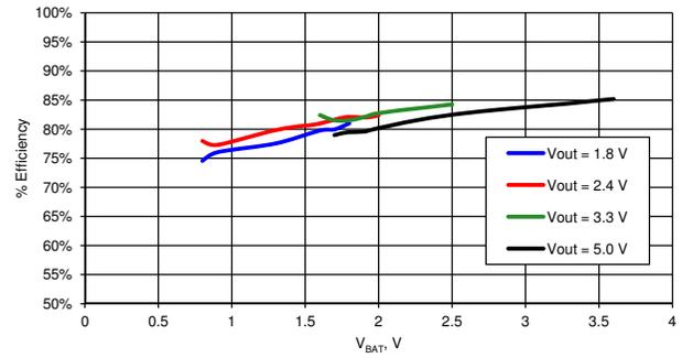
**Figure 11-13. Efficiency vs  $V_{BAT}$ ,  $L_{BOOST} = 22 \mu H$  [38]**
