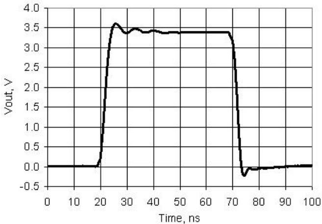
**Figure 11-21. SIO Output Rise and Fall Times, Slow Strong Mode, V<sub>DDIO</sub> = 3.3 V, 25 pF Load**
