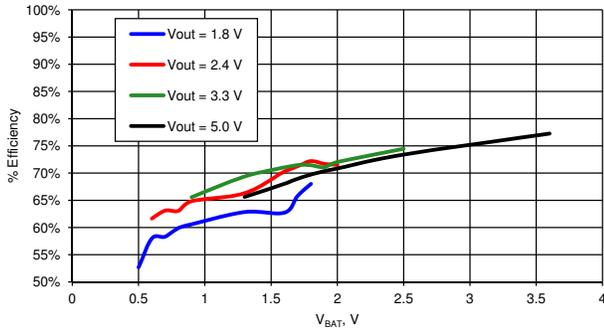
**Figure 11-12. Efficiency vs  $V_{BAT}$ ,  $L_{BOOST} = 10 \mu H$  [38]**
