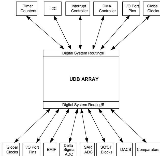
Interrupt and DMA routing is very flexible in the CY8C38 programmable architecture. In addition to the numerous fixed function peripherals that can generate interrupt requests, any data signal in the UDB array routing can also be used to generate a request. A single peripheral may generate multiple independent interrupt requests simplifying system and firmware design. Figure 7-10 shows the structure of the IDMUX (Interrupt/DMA Multiplexer).
