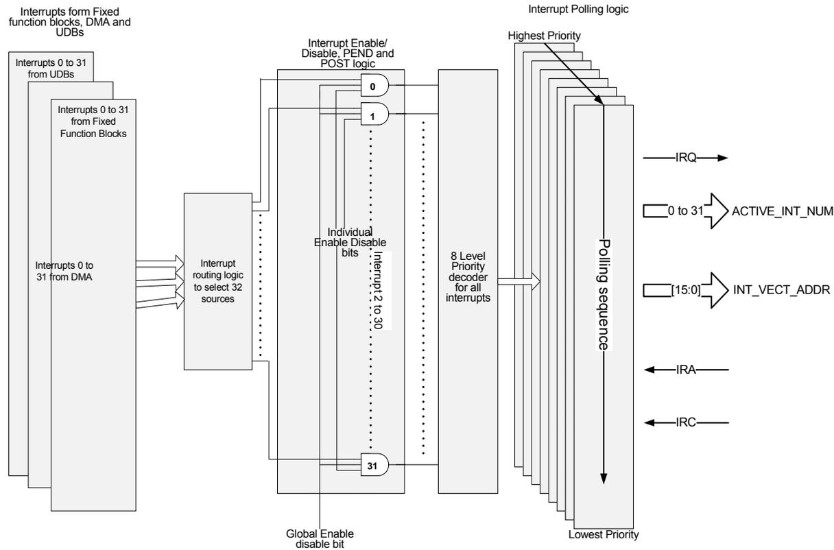
When an interrupt is pending, the current instruction is completed and the program counter is pushed onto the stack. Code execution then jumps to the program address provided by the vector. After the ISR is completed, a RETI instruction is executed and returns execution to the instruction following the previously interrupted instruction. To do this the RETI instruction pops the program counter from the stack.
