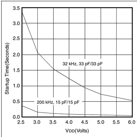
**FIGURE 23-24: TYPICAL XTAL STARTUP TIME vs. VDD (XT MODE, 25°C)**
