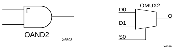
Figure 20: AND & MUX Symbols in XC4000X IOB
