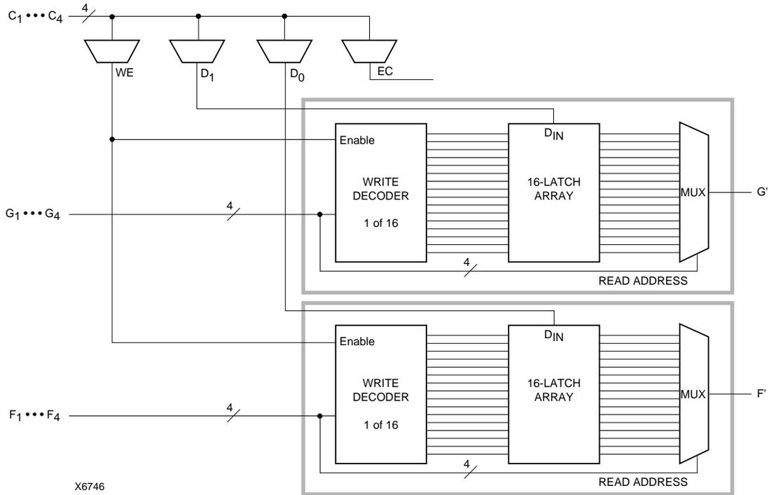
Figure 9: 16x2 (or 16x1) Level-Sensitive Single-Port RAM
