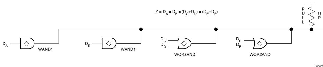
**Figure 21: Open-Drain Buffers Implement a Wired-AND Function**
