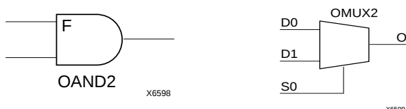
Figure 20: AND & MUX Symbols in XC4000X IOB
