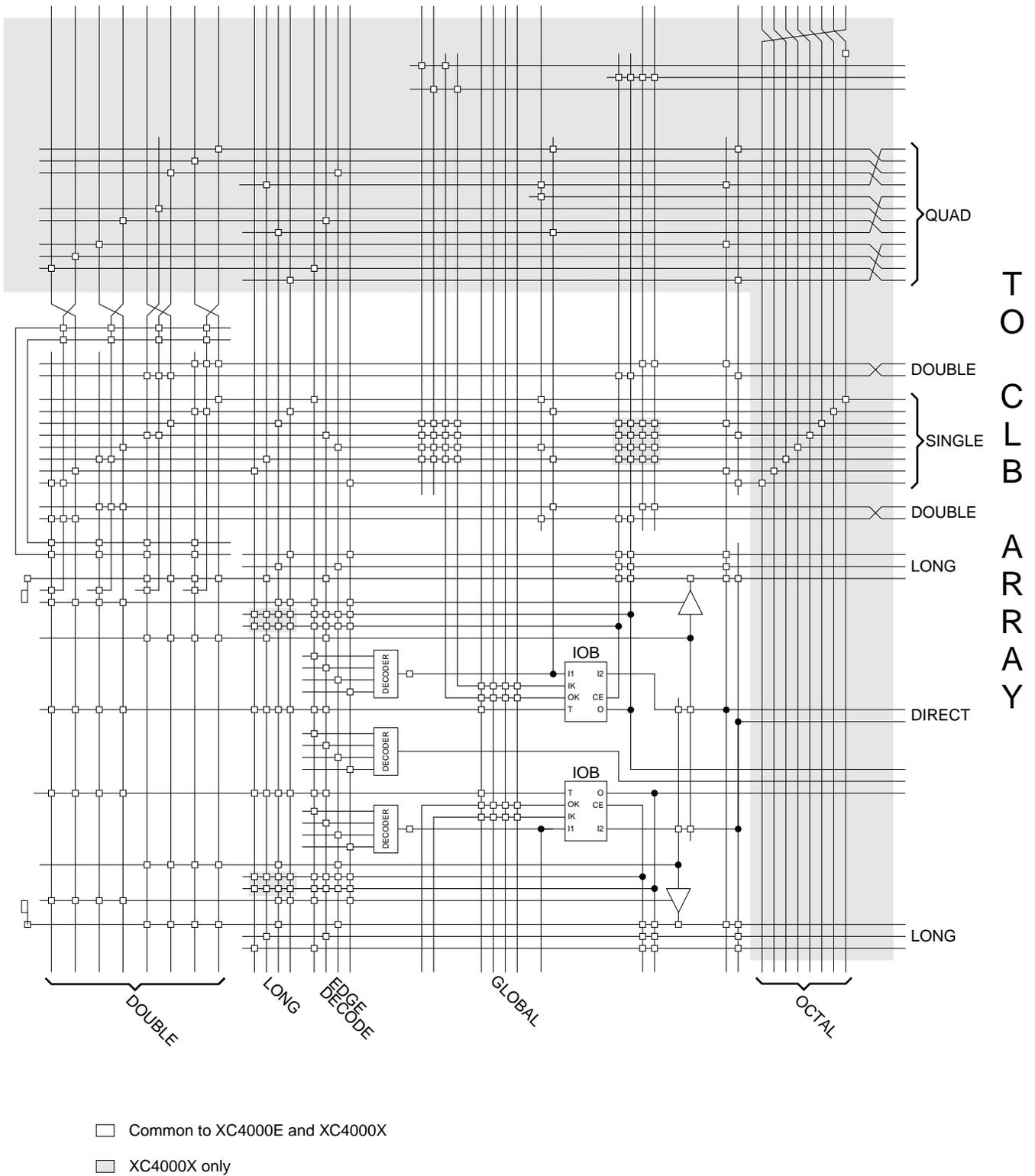
IOB inputs and outputs interface with the octal lines via the single-length interconnect lines. Single-length lines are also used for communication between the octals and double-length lines, quads, and longlines within the CLB array.
