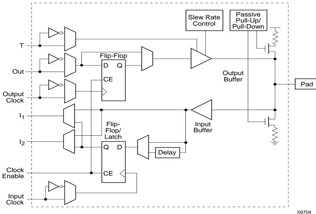
Figure 15: Simplified Block Diagram of XC4000E IOB
