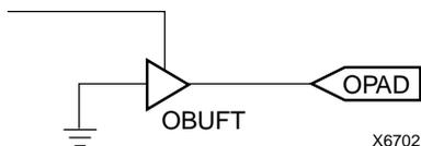
**Figure 18: Open-Drain Output**
