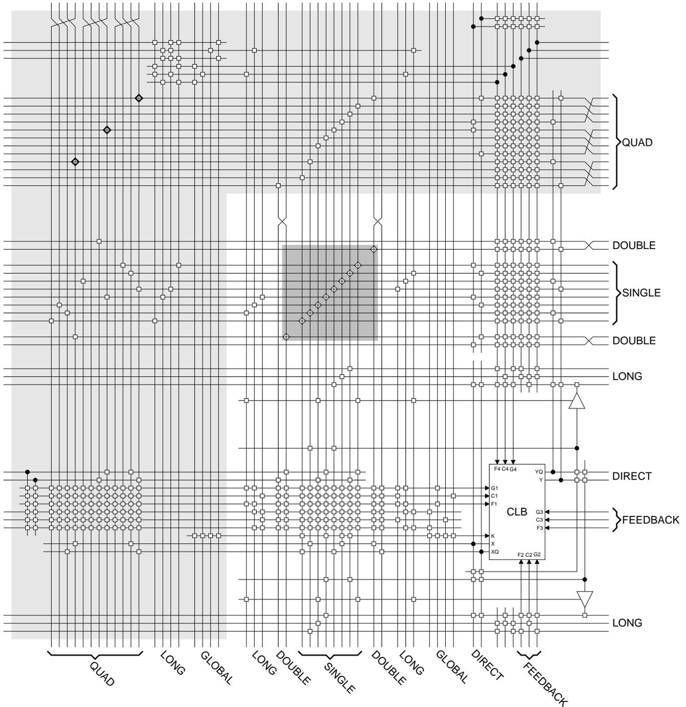
**Figure 27: Detail of Programmable Interconnect Associated with XC4000 Series CLB**
