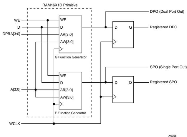
**Figure 6: XC4000 Series Dual-Port RAM, Simple Model**
