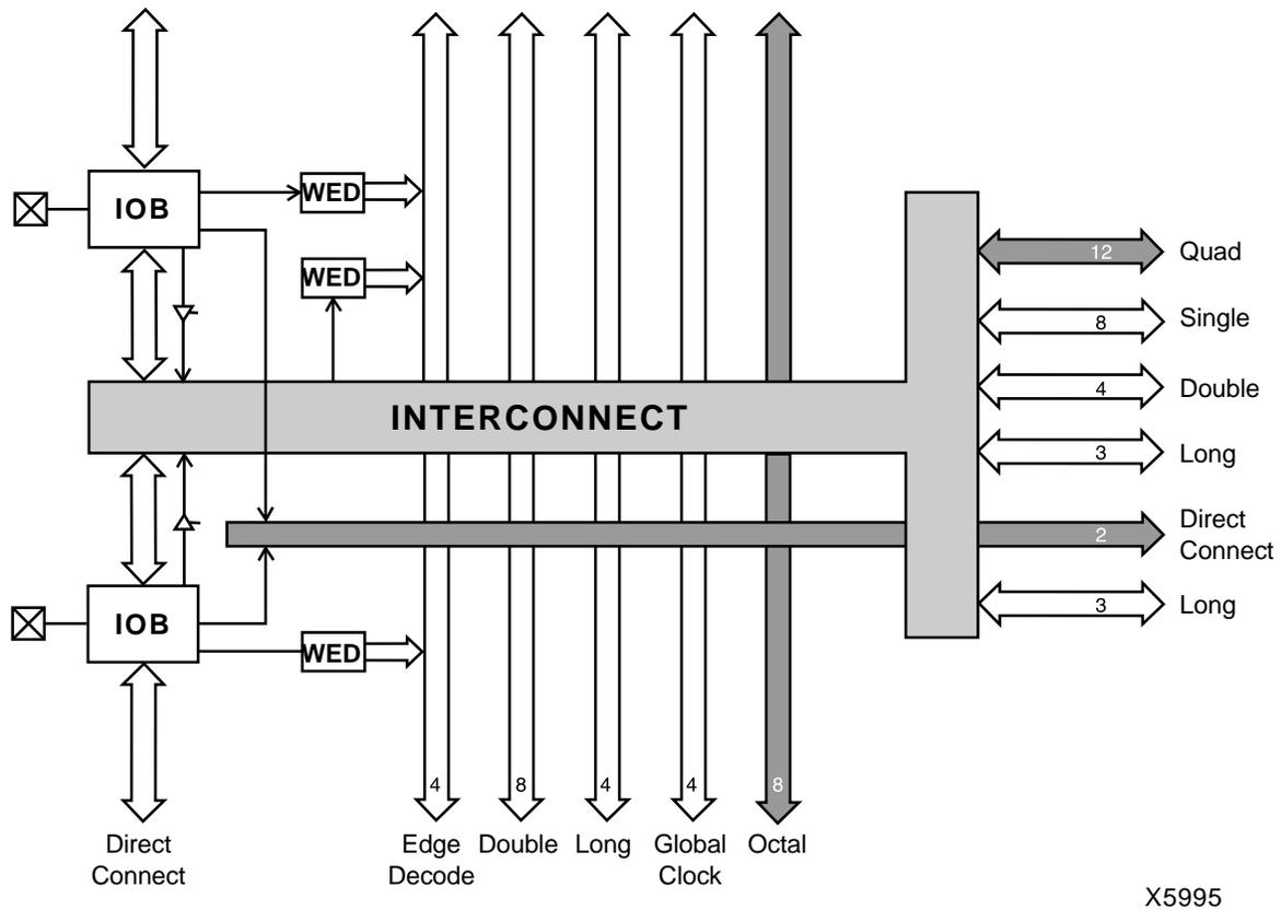
Figure 31: High-Level Routing Diagram of XC4000 Series VersaRing (Left Edge)
