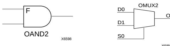
Figure 20: AND & MUX Symbols in XC4000X IOB
