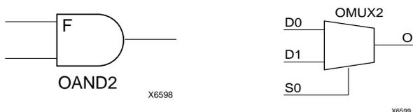
**Figure 20: AND & MUX Symbols in XC4000X IOB**
