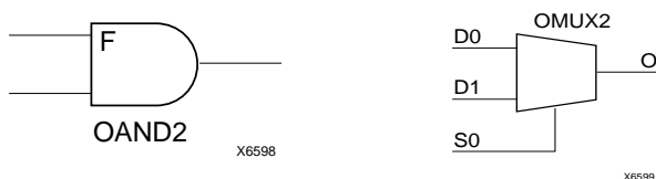
Figure 20: AND & MUX Symbols in XC4000X IOB
