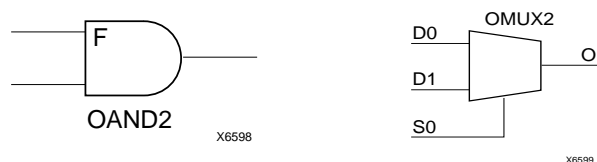
Figure 20: AND & MUX Symbols in XC4000X IOB
