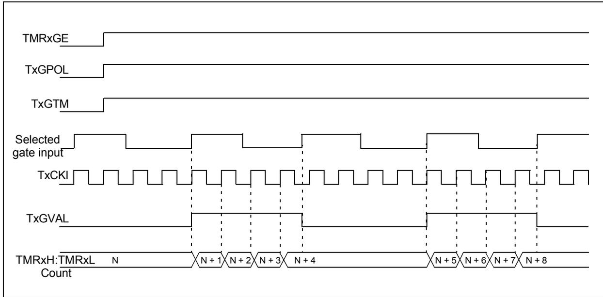
**FIGURE 26-5: TIMER1 GATE SINGLE-PULSE MODE**
