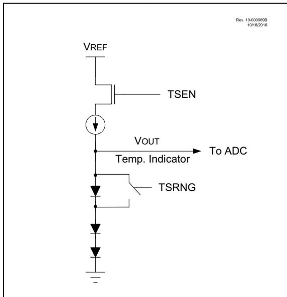
The output of the circuit is measured using the internal Analog-to-Digital Converter. A channel is reserved for the temperature circuit output. Refer to **Section 20.0 “Analog-to-Digital Converter (ADC) Module”** for detailed information.
