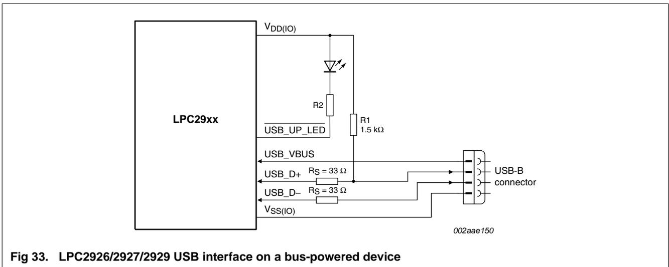
Fig 33. LPC2926/2927/2929 USB interface on a bus-powered device
