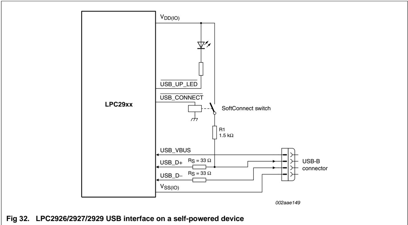
Fig 32. LPC2926/2927/2929 USB interface on a self-powered device
