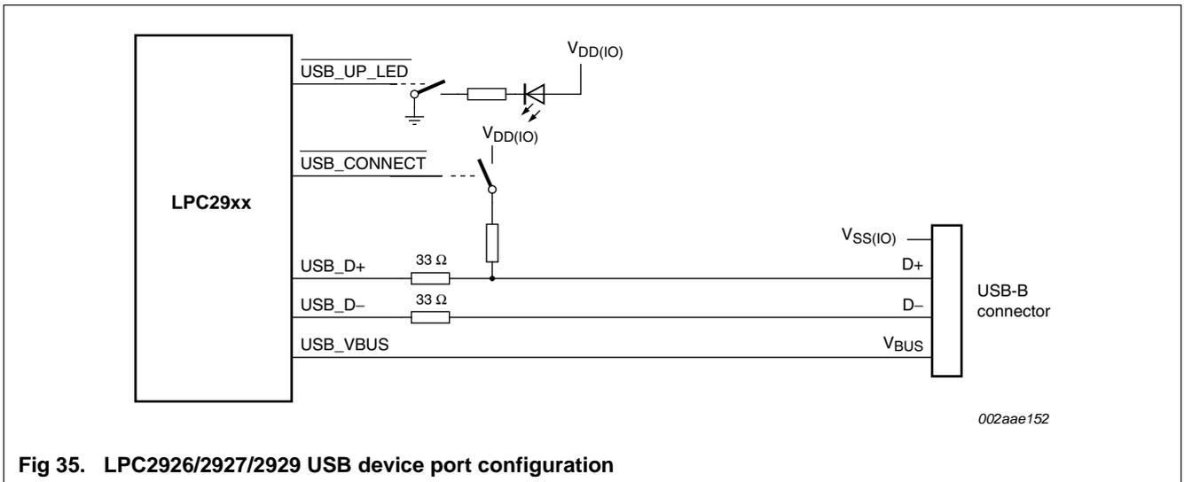
**Fig 35. LPC2926/2927/2929 USB device port configuration**
