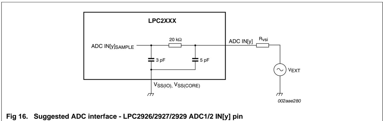
**Fig 16. Suggested ADC interface - LPC2926/2927/2929 ADC1/2 IN[y] pin**
