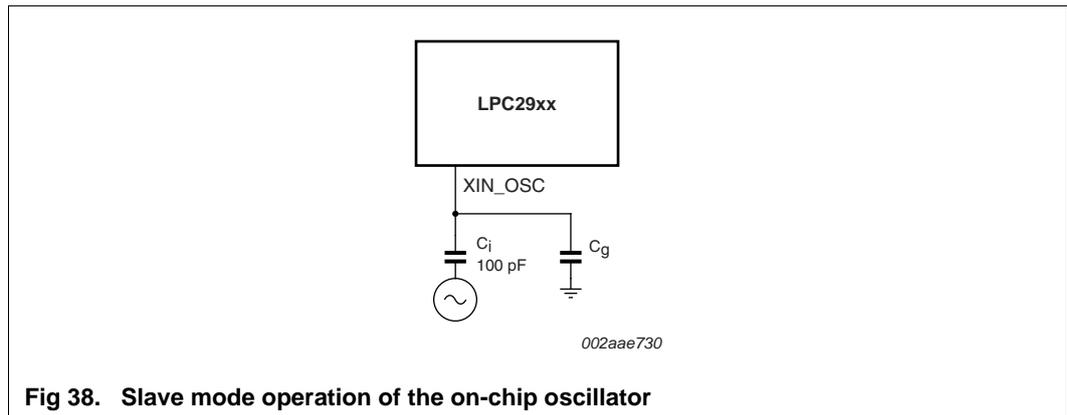
Fig 38. Slave mode operation of the on-chip oscillator
