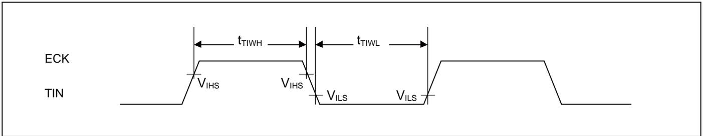
**Trigger input timing**
