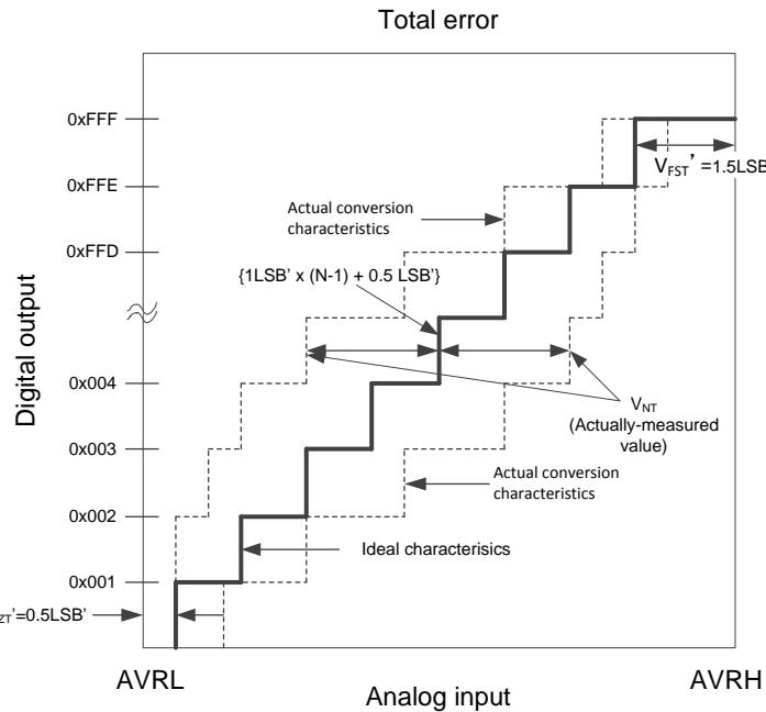
$$\text{Total error of digital output } N = \frac{V_{NT} - \{1 \text{ LSB}' \times (N-1) + 0.5 \text{ LSB}'\}}{1 \text{ LSB}'} \quad [\text{LSB}]$$
