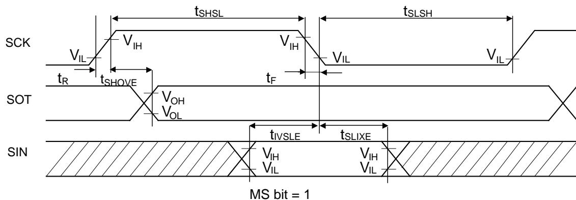
**When Using High-Speed Synchronous Serial Chip Select (SCINV = 0, CSLVL = 0)**
