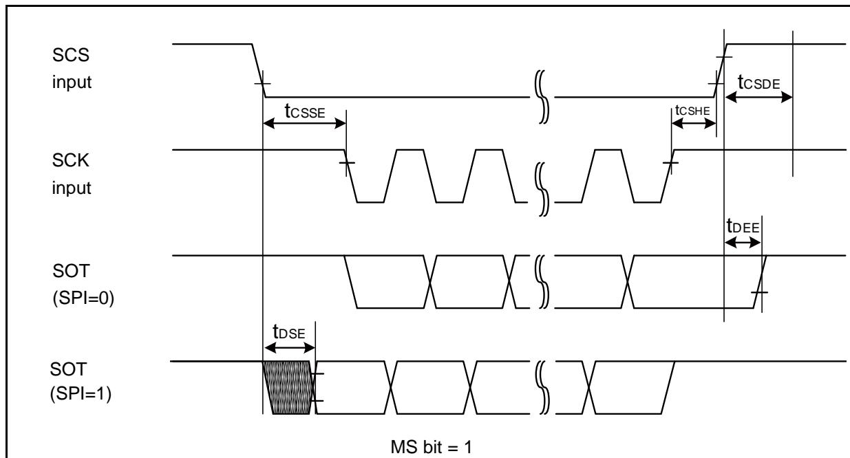
**High-Speed Synchronous Serial (SPI = 0, SCINV = 1)**
