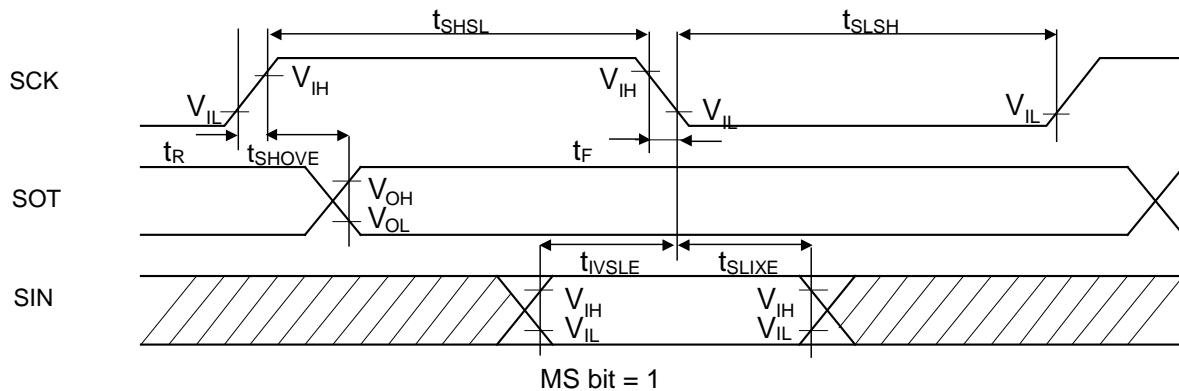
**When Using Synchronous Serial Chip Select (SCINV = 0, CSLVL = 0)**
