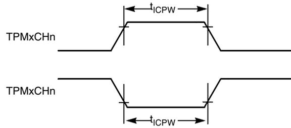
**Figure 3-14. Timer Input Capture Pulse**
