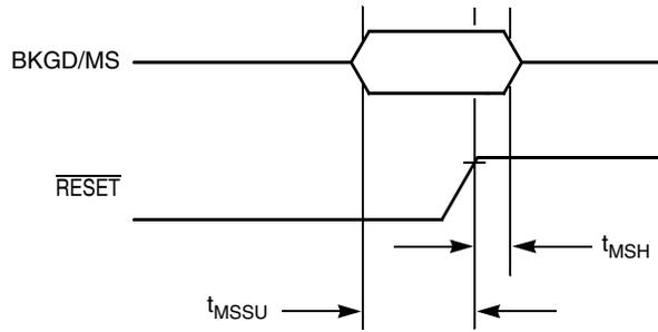
Figure 3-11. Active Background Debug Mode Latch Timing
