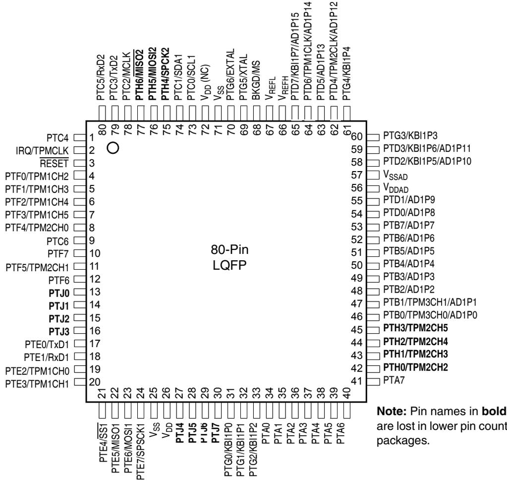
Figure 2-1. MC9S08AC128 Series in 80-Pin LQFP Package
