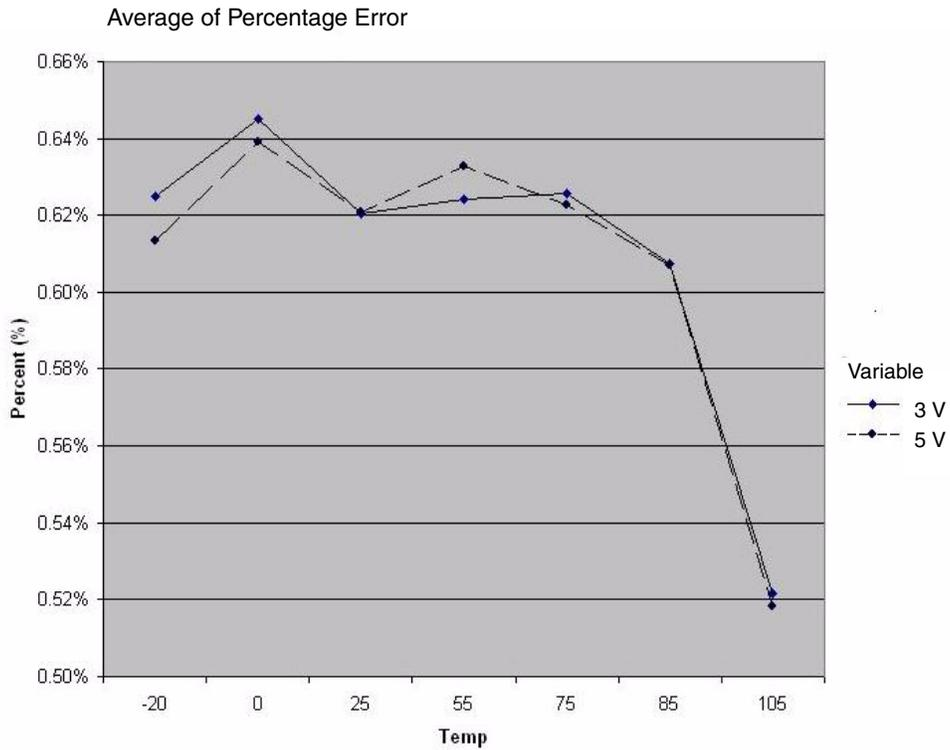
**Figure 3-9. Internal Oscillator Deviation from Trimmed Frequency**
