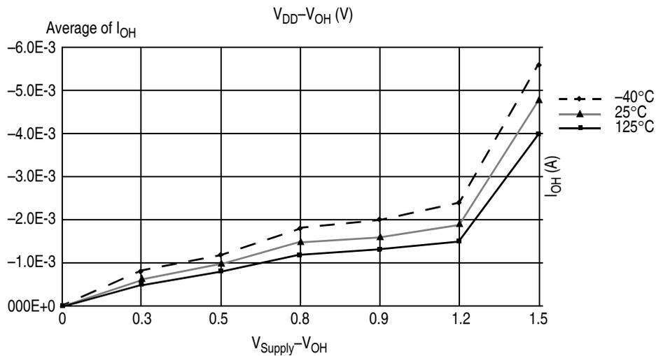
**Figure 3-1. Typical I<sub>OH</sub> (Low Drive) vs V<sub>DD</sub>-V<sub>OH</sub> at V<sub>DD</sub> = 3 V**
