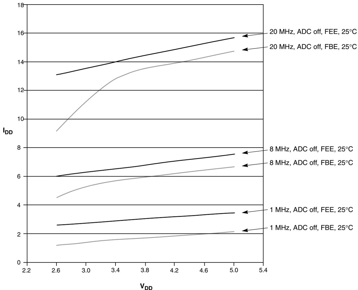
Note: External clock is square wave supplied by function generator. For FEE mode, external reference frequency is 4 MHz
