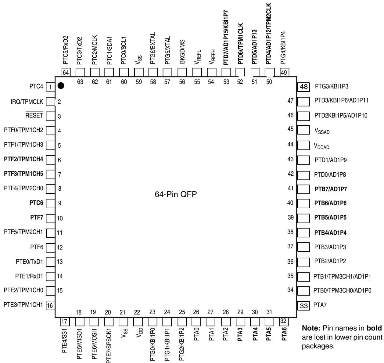
Figure 2-2. MC9S08AC128 Series in 64-Pin QFP Package
