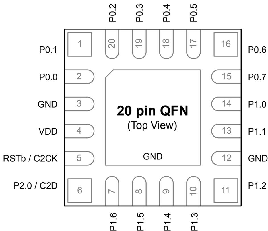
Figure 6.3. EFM8BB2x-QFN20 Pinout
