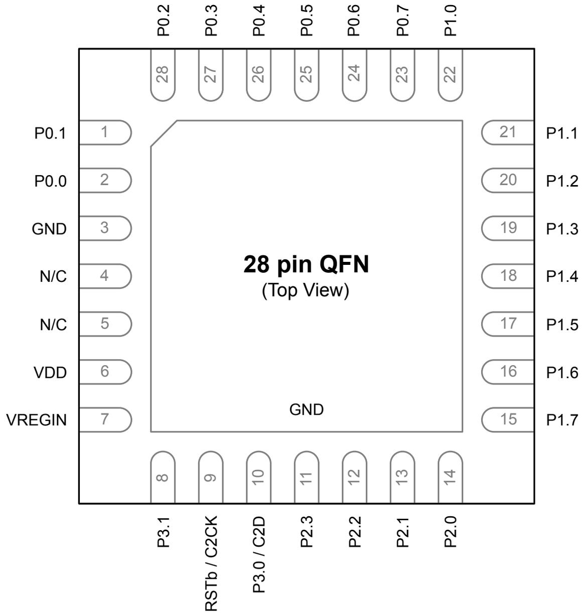
Figure 6.1. EFM8BB2x-QFN28 Pinout
