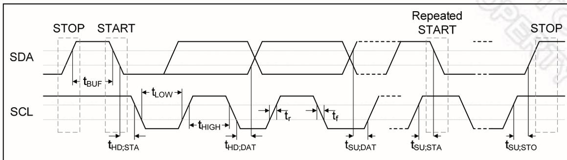
Figure 5-9 I<sup>2</sup>C Bus Timing
