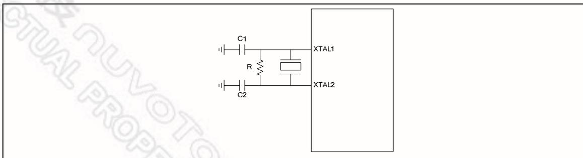
Figure 7-1 Typical Crystal Application Circuit
