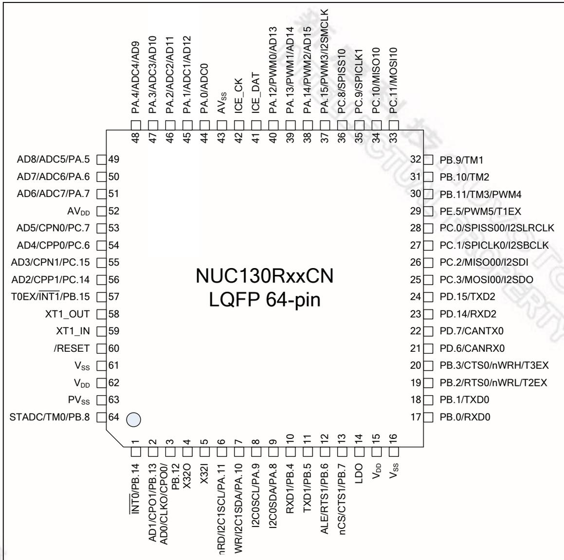
Figure 3-3 NuMicro™ NUC130 LQFP 64-pin Pin Diagram
