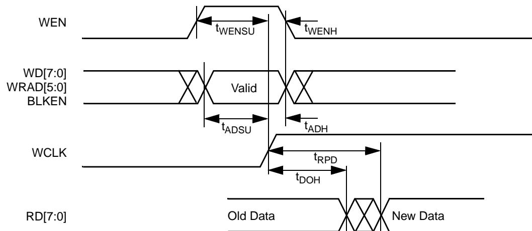
**A1240A Timing Characteristics**(Worst-Case Military Conditions,  $V_{CC} = 4.5V$ ,  $T_J = 125^{\circ}C$ )
