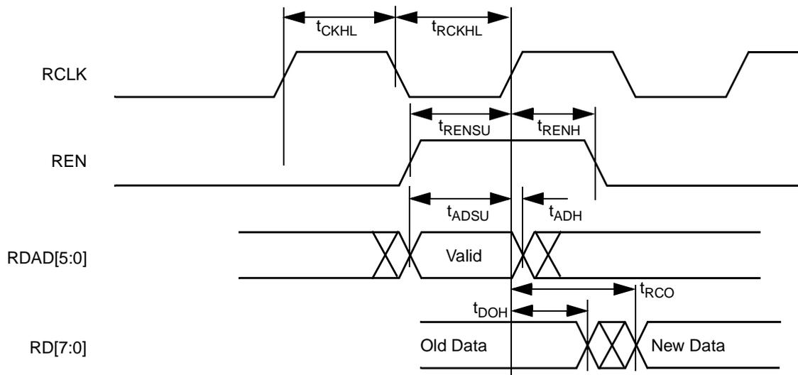
*Note: Identical timing for falling-edge clock.*
