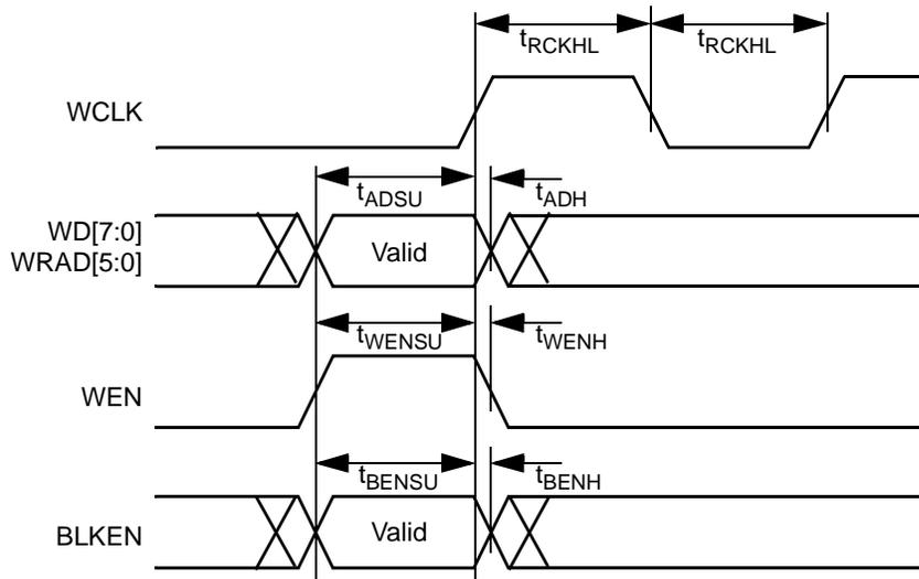
*Note: Identical timing for falling-edge clock.*
