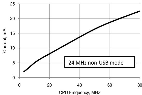
**Figure 11-2.  $I_{DD}$  vs Frequency at  $25\text{ }^{\circ}\text{C}$**
