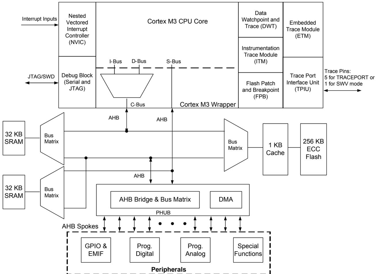
The Cortex-M3 CPU subsystem includes these features:
