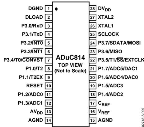
Figure 2. Pin Configuration
