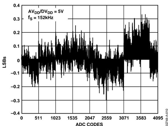
Figure 3. Typical INL Error,  $V_{DD} = 5 V$
